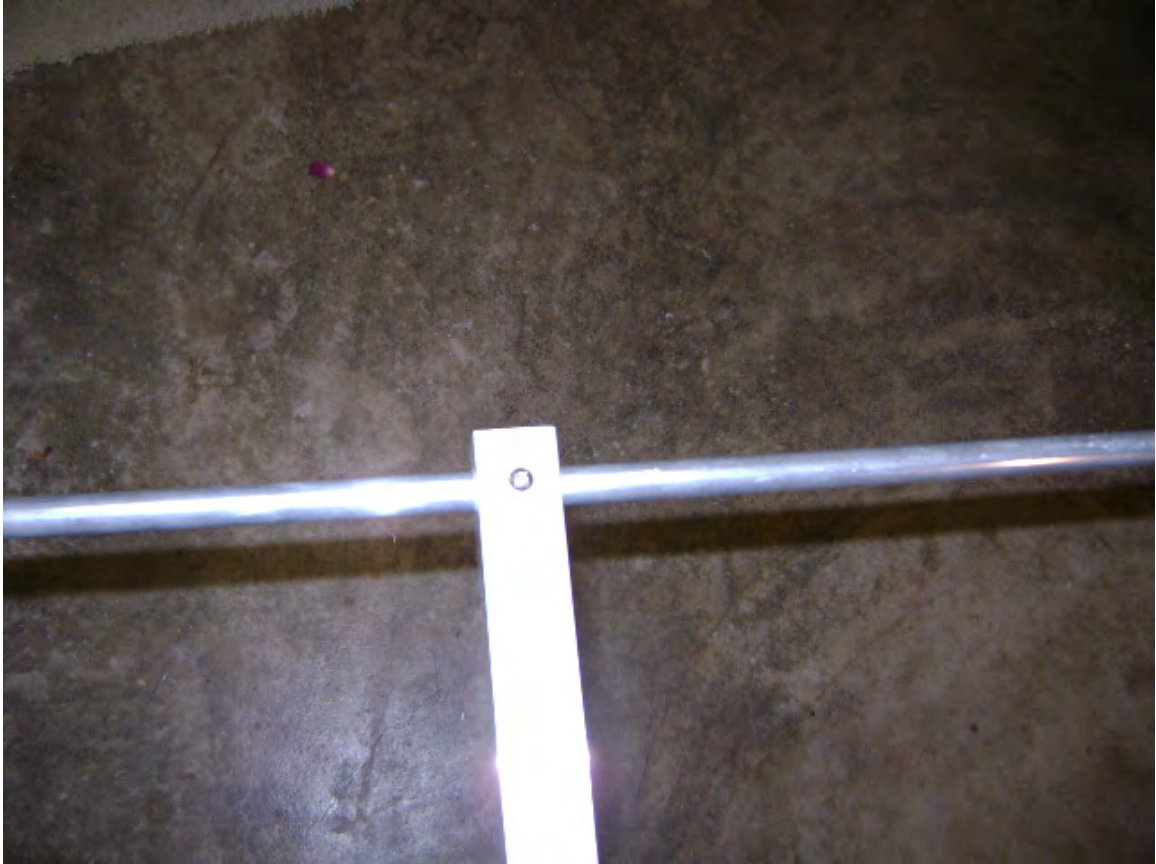
Figure 2. Center Elements into Boom Installation
